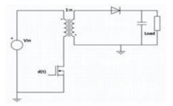
When the switch, generally a power MOSFET, turns on, the transformer is energized. The relationship of the transformer's input voltage to its output voltage is determined by its windings ratio. The "dots" on the wirings of the transformer indicate that a positive voltage on the input wiring means a negative voltage will appear on the secondary. Thus, the diode will be reverse-biased, so no current flows, but a magnetic field is created in the primary (input) coil's windings.
