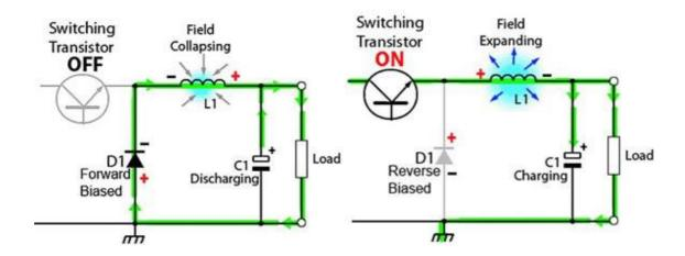
The diagram above is a highly simplified diagram of a buck converter. When the "switch," usually a power MOSFET/TRANSISTOR, is turned on, voltage in the inductor (L1) is generated that opposes the voltage from the source. Thus, voltage across the load and capacitor (C1) never gets as high as the input voltage from the source.
