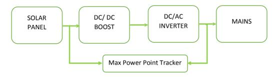
There are three main stages in conversion of DC to AC of Solar inverter:-
